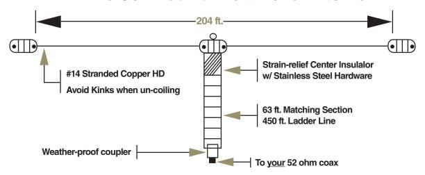
This antenna should be supported with rope or other non-conductor.
